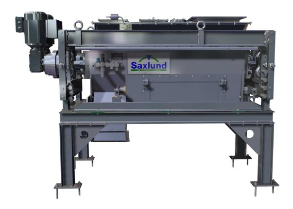
The Saxlund coarse material separator protects your system by removing any unwanted objects from the infeed material. By separating out the contaminants that are too large for further processing, there is less damage done to your plant machinery and a higher prevention of failures further downstream.
