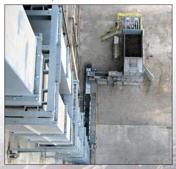
Protecting the environment while lowering operating costs is a challenge to be met. Reducing specific fuel requirements and switching from wet to dry processes has already resulted in significant improvements in energy efficiency. Procedural innovations in the field of highly automated conveyor technology ensure a constant production and exact metering of the fuels.
